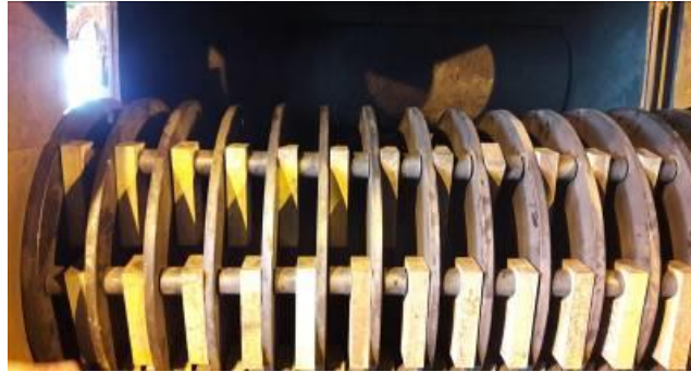
Fig. 2. Crushers drills in idle position
