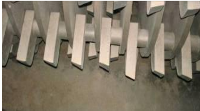
Fig. 4. Uneven wear-out of the hammer along the axis or width of the rotor
