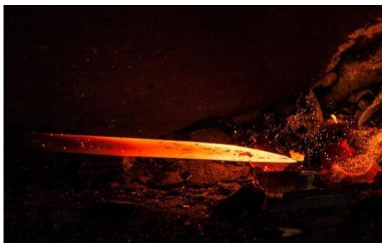
Fig. 2. Partially heated up end of a part to be forged a) and air supplying into forging fire b)
