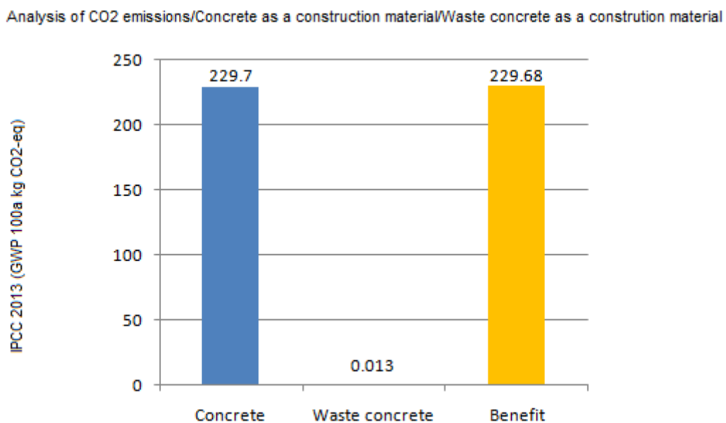
Fig. 3. Analysis of kg CO 2 emissions using concrete as construction materials and using waste concrete in the construction processes [4]
