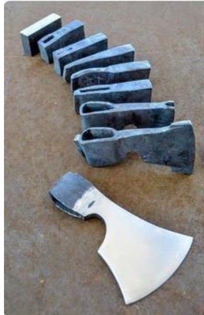
Fig. 6. Some steps in hand forging/forge welding of an axe with insert of high carbon steel
