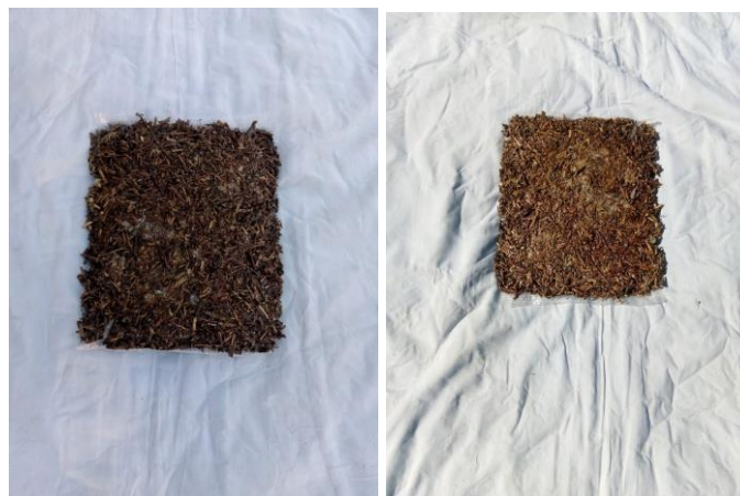
Fig. 11. Appearance of thermosonic insulation boards for the needs of the company "Drvo-Art" from Čačak.
