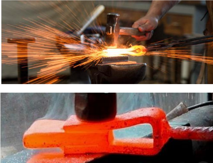
Fig. 4. Critical moments in hand forge welding: a) beginning (bright color) and b) at the end (pieces were cooled to orange color)
