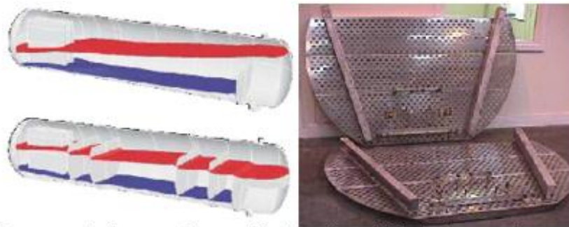
Fig. 4. Influence of barriers on liquid rolling and barrier appearance [1]
