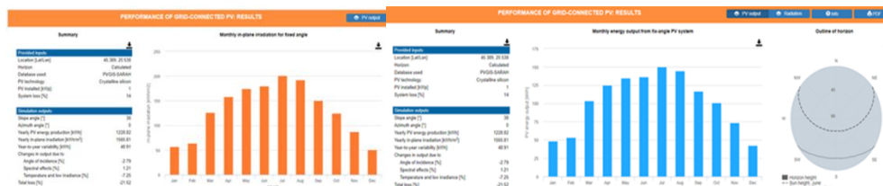
Fig. 5. Simulation of monthly radiation in plane with PV panel and simulation of generated energy with fixed angle of PV panel
